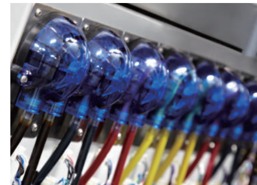
Peristaltic-pump ink supply
