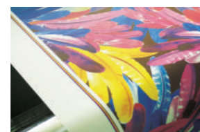
Dye sublimation transfer paper printing
